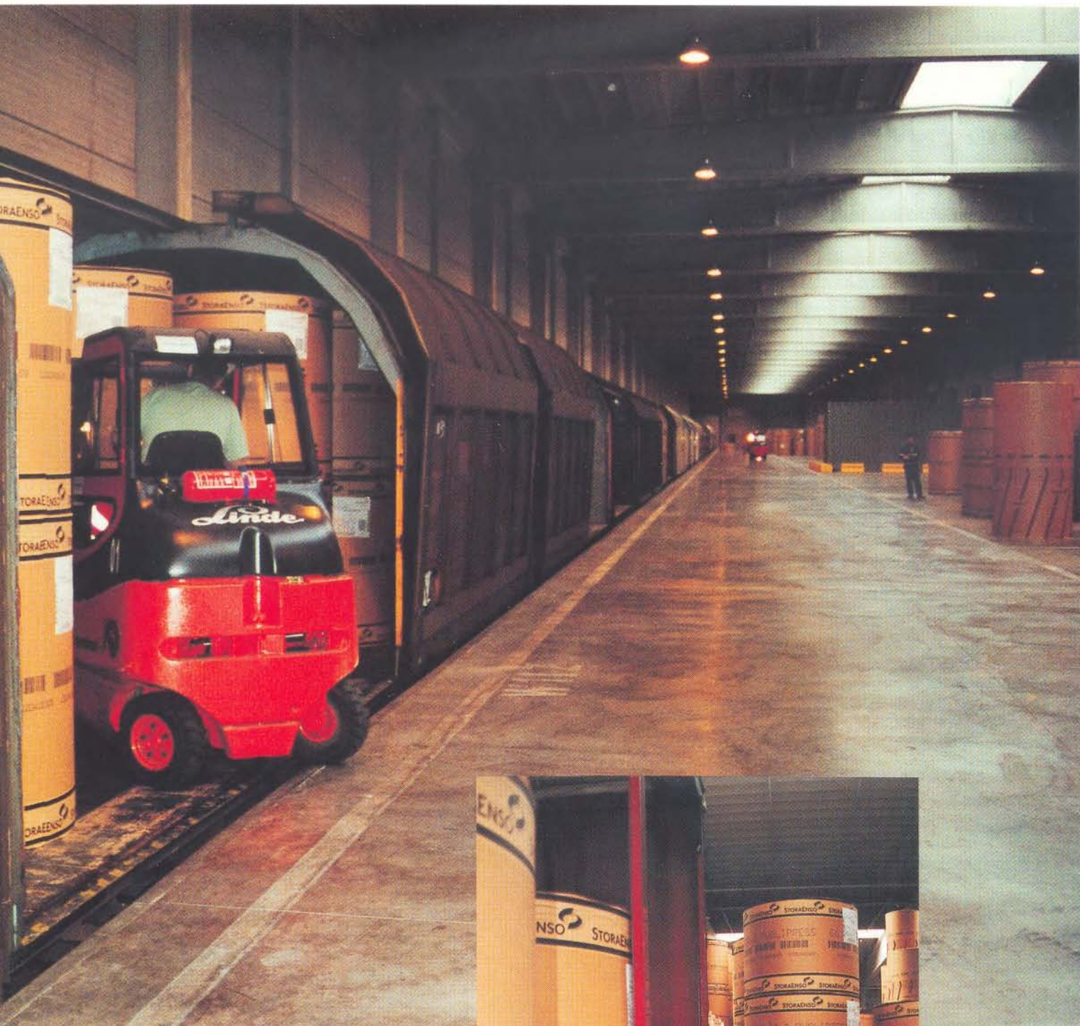
Cross docking from SECUs to rail cars is conducted using electrically powered "grabber" trucks.
